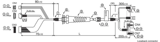
When connecting to an OMRON PLC, the control signals must be looped back. Connect loopback connectors to CN8 and CN7.
