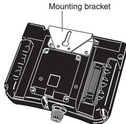
**Note:** Tighten the screws to a force of 0.9 N·m.
